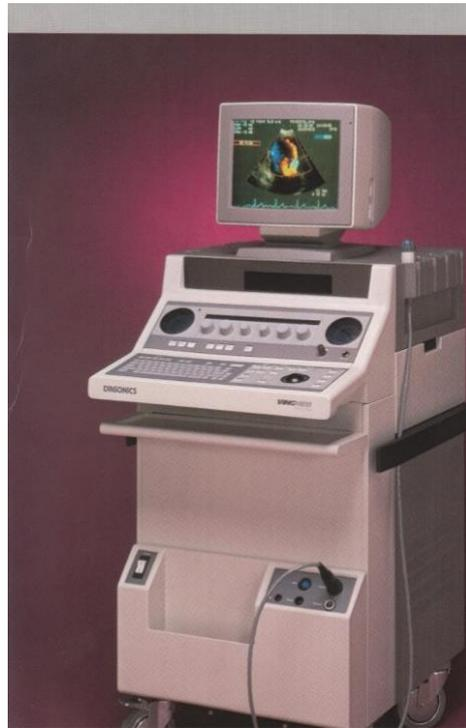
**Figure 3** System 5. The first ultrasound scanner from Vingmed with electronic probes.
