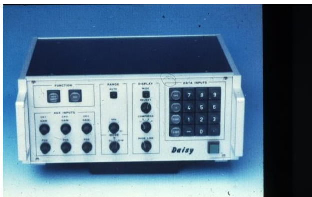
Figure 3 DAISY. The first commercially available real-time spectral-analyzer
