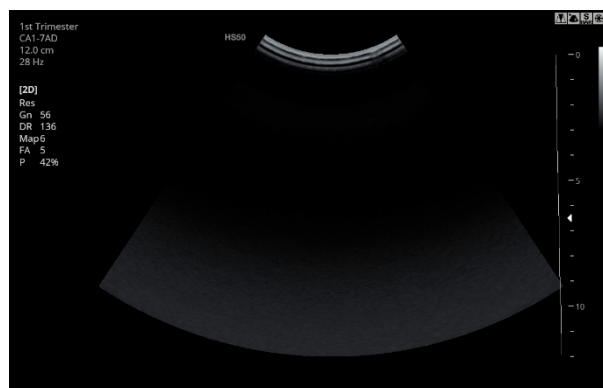
Figure 18 Subtle, focal inhomogeneity of the reverberation lines on the left, but no defect (10).
