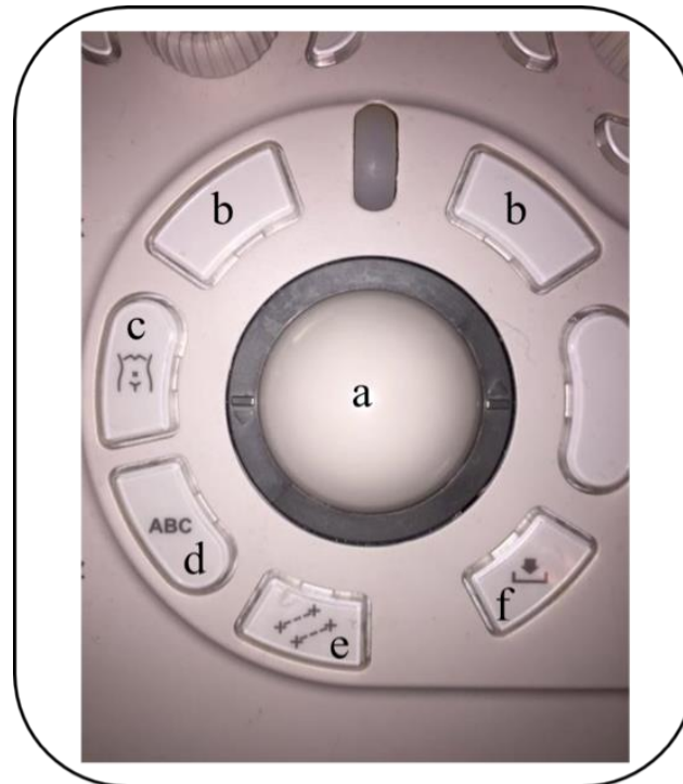
Figure 7 Example of layout of function keys/symbols for ease of use – a. trackball, b. unlabelled 'select' keys, c. body marker, d. text annotation, e. measurement callipers, f. storage.
